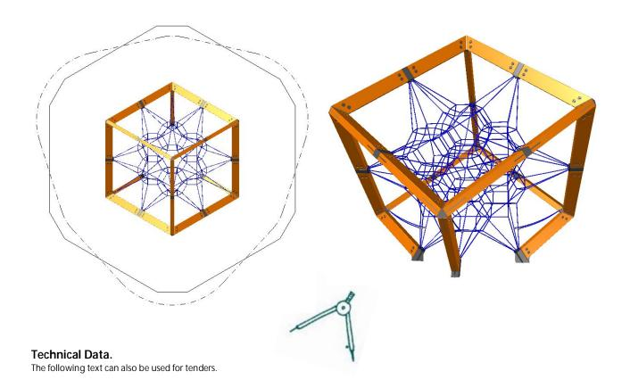
Climbing Cube "The Cube" from the Joe Brown Collection, consisting of a larch timber structure with a 12-fold Spacial net, equipped with the ASTEM TT tension system concealed in the containers for clamping the spatial net. The foundation parts made of powder-coated steel, fitted into the wood elements, ensure the installation of the support members without direct involvement of the bottom timber carrier with the ground.
